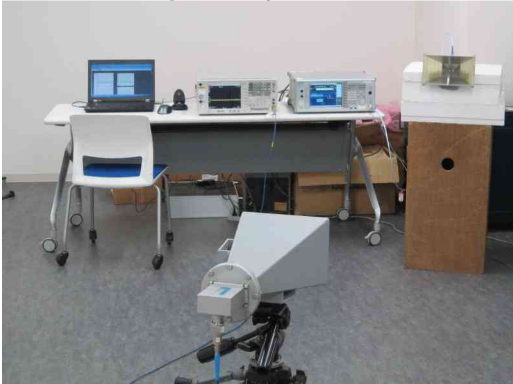
Test Setup for Generating the Radar Waveform
