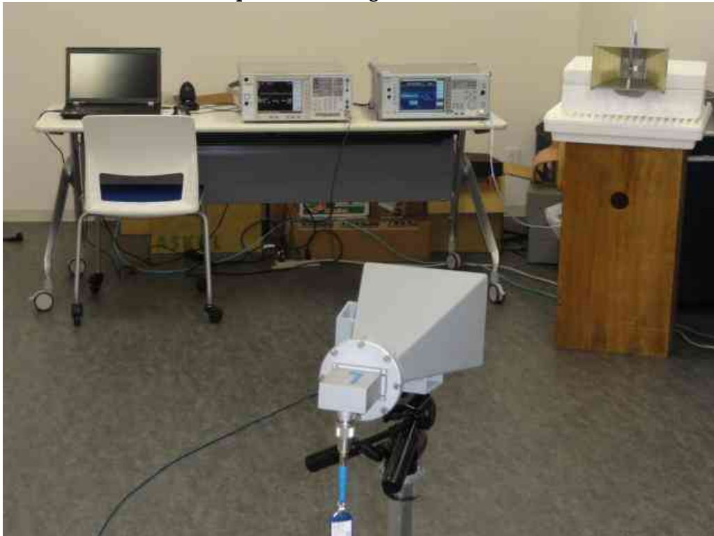
Test Setup for Generating the Radar Waveform
