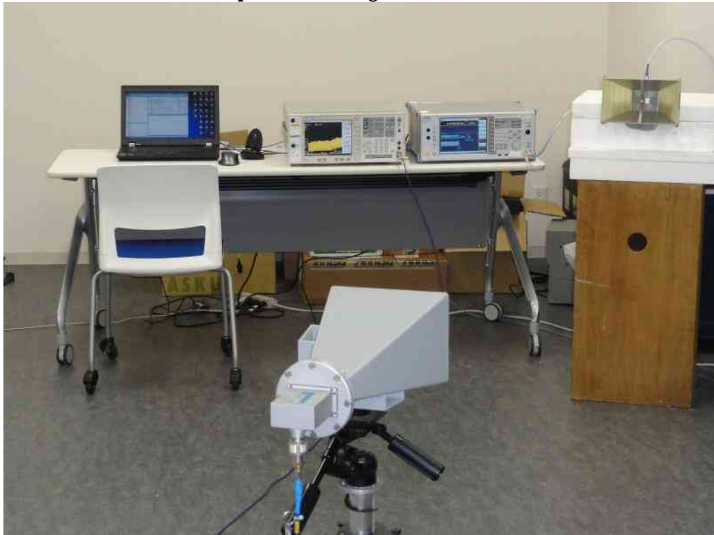
Test Setup for Generating the Radar Waveform
