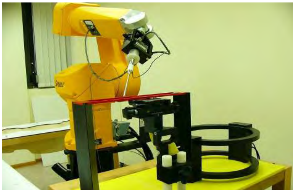
Fig. 1 Photograph of the DASY 5 measurement system
