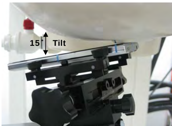
Fig.6 Left Head Section / Ear-Tilt Position(15°)
