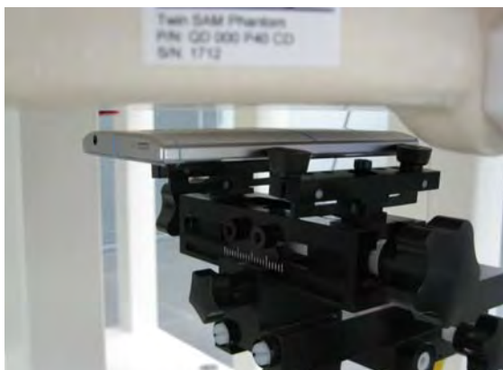
Fig.10 EUT back side to flat phantom
