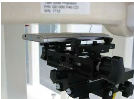
Fig.8 EUT back side to flat phantom
