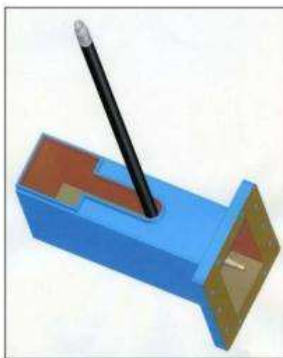
Figure 4. Schematic showing the innovative design of slot in the waveguide termination
