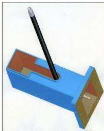
Figure 2 Schematic showing the innovative design of slot in the waveguide termination
