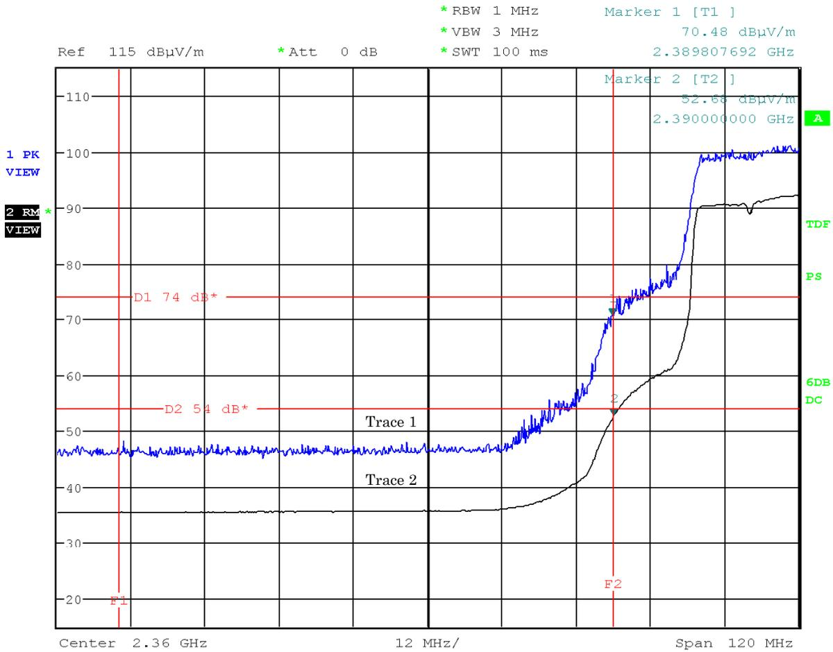
Note: The trace 1 is Peak detection. The trace 2 is RMS detection.
