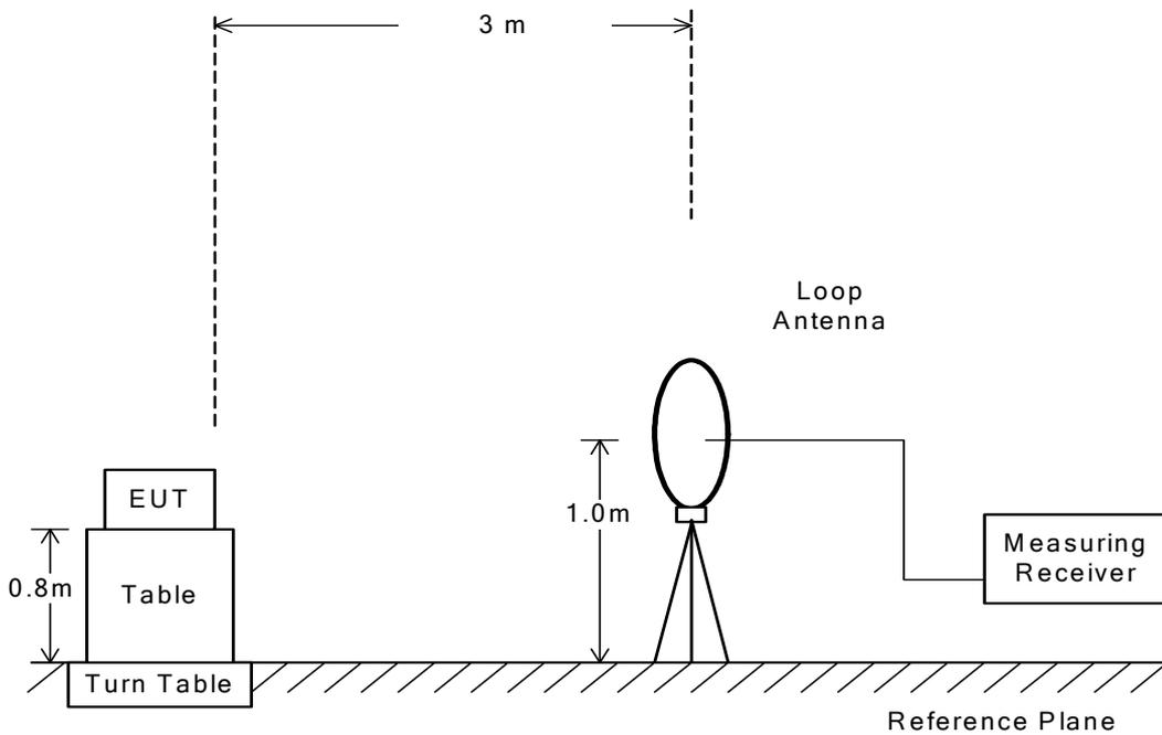
**7.9.4.2 Radiated Emission 30 MHz – 1000 MHz**
