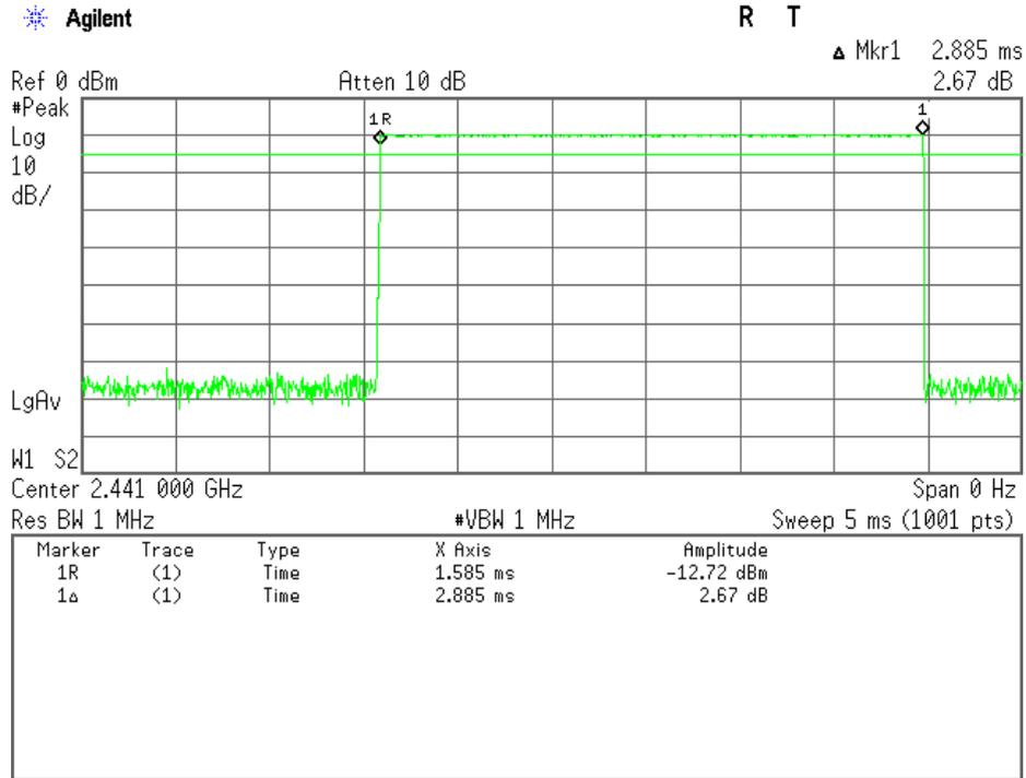
Note : A DH5 Packet need 5 time slot for transmitting and 1 time slot for receiving. Then the system makes worst case 266.667 hops per second with 79 channels. So the system have each channel 3.3755 times per second and so for 31.6 seconds the system have 106.7 times of appearance. Each tx-time per appearance is 2.885 ms.
