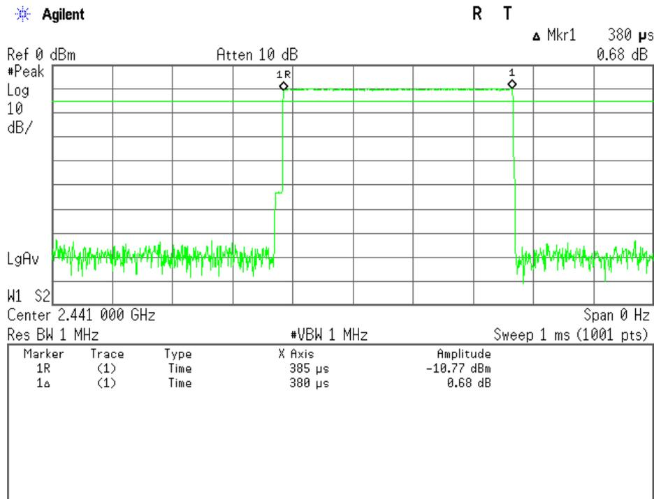
Note : The system makes worst case 1600 hops per second or 1 time slot has a length of 625 μs with 79 channels. A DH1 Packet need 1 time slot for transmitting and 1 time slot for receiving. Then the system makes worst case 800 hops per second with 79 channels. So the system has each channel 10.1266 times per second and so for 31.6 seconds the system have 320.0 times of appearance.
