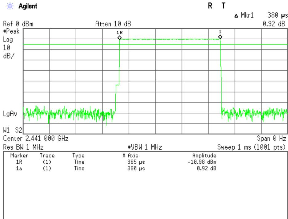
Note : The system makes worst case 1600 hops per second or 1 time slot has a length of 625 μs with 79 channels. A DH1 Packet need 1 time slot for transmitting and 1 time slot for receiving. Then the system makes worst case 800 hops per second with 20 channels. So the system has each channel 40 times per second and so for 8 seconds the system have 320.0 times of appearance.
