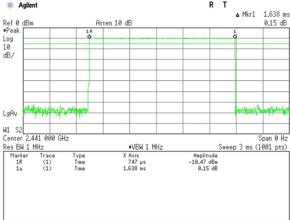
Note : A DH3 Packet need 3 time slot for transmitting and 1 time slot for receiving. Then the system makes worst case 400 hops per second with 20 channels. So the system have each channel 20 times per second and so for 8 seconds the system have 160.0 times of appearance. Each tx-time per appearance is 1.638 ms. Dwell time = 160.0 \* 1.638 = 262.1 ms
