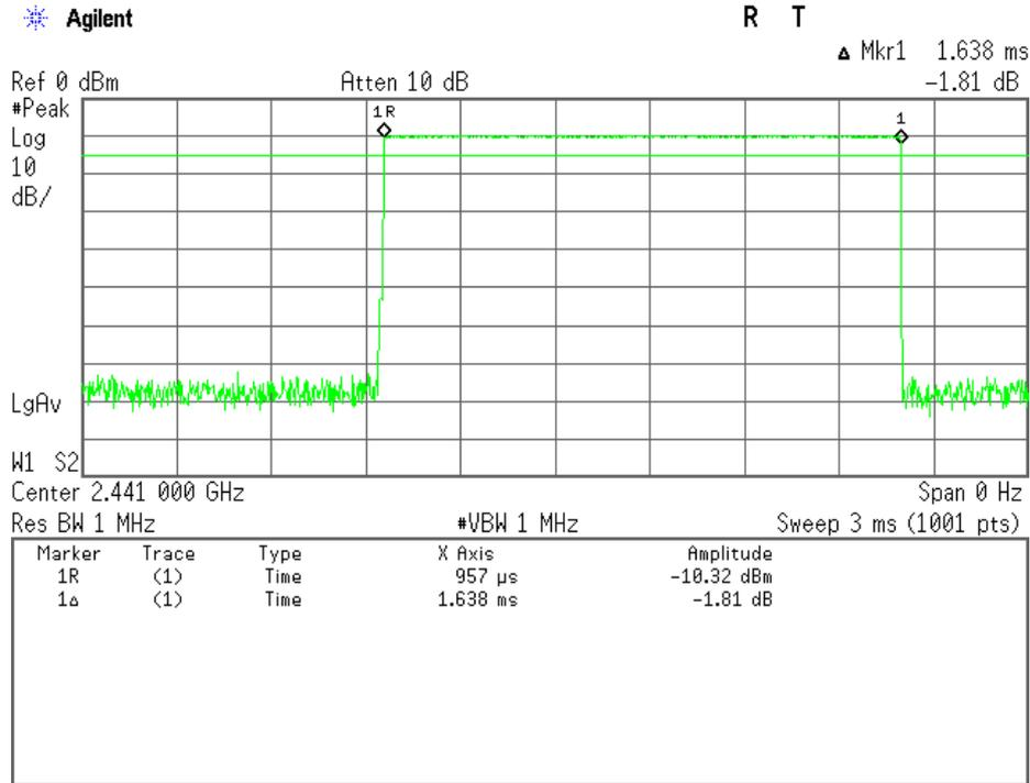
Note : A DH3 Packet need 3 time slot for transmitting and 1 time slot for receiving. Then the system makes worst case 400 hops per second with 79 channels. So the system have each channel 5.063 times per second and so for 31.6 seconds the system have 160.0 times of appearance. Each tx-time per appearance is 1.638 ms.
