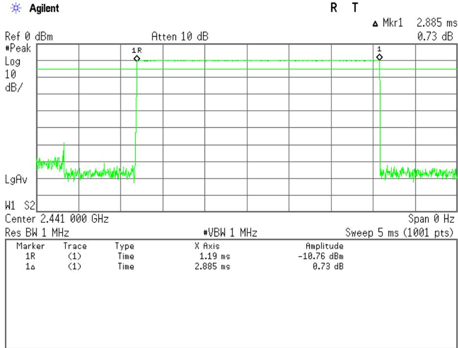
Note : A DH5 Packet need 5 time slot for transmitting and 1 time slot for receiving. Then the system makes worst case 266.667 hops per second with 20 channels. So the system have each channel 13.33335 times per second and so for 8 seconds the system have 106.7 times of appearance. Each tx-time per appearance is 2.885 ms.
