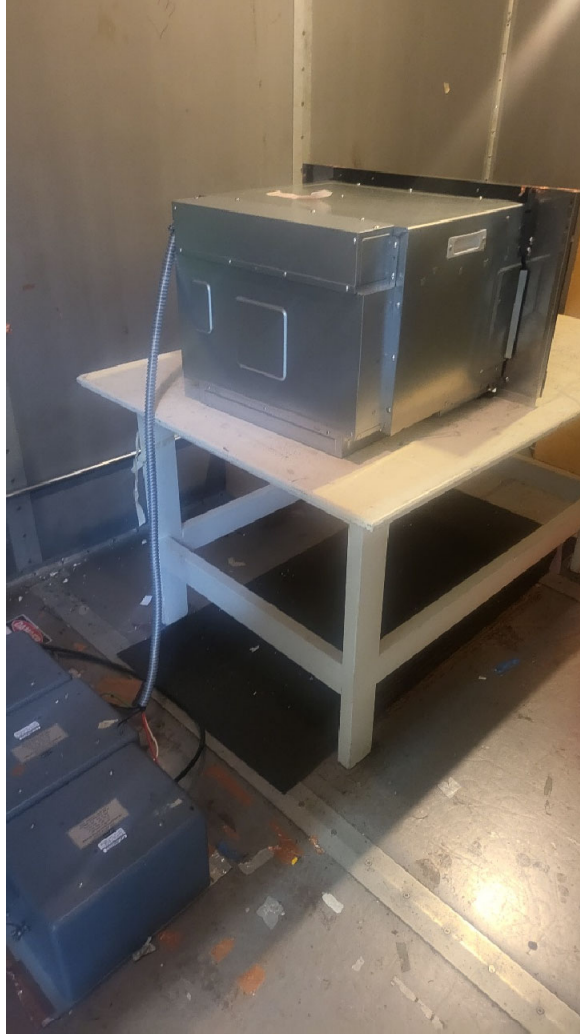
Figure 8. Photograph of Conducted Emissions Test Configuration
