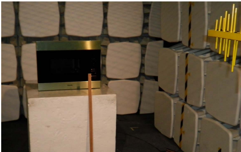
Photograph 5.7.2 Radiated emissions testing 30MHz-1GHz (Anechoic chamber)
