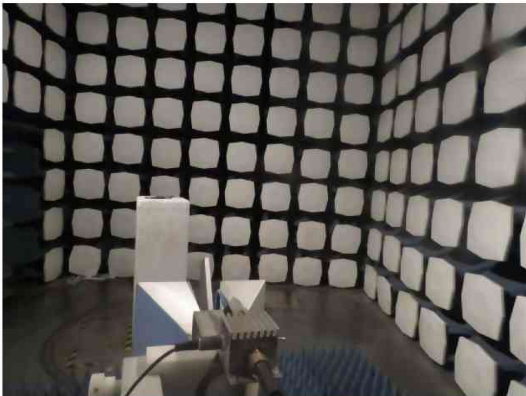
Picture 2: Radiated Spurious Emissions Test setup
