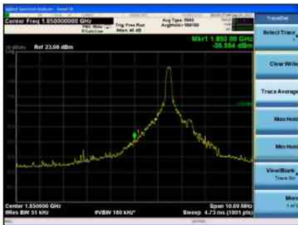
LTE Band 2 20MHz 16QAM 100%RB CH-Low
