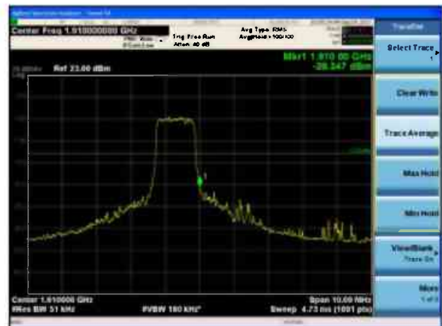
LTE Band 2 3MHz QPSK 1RB CH-High
