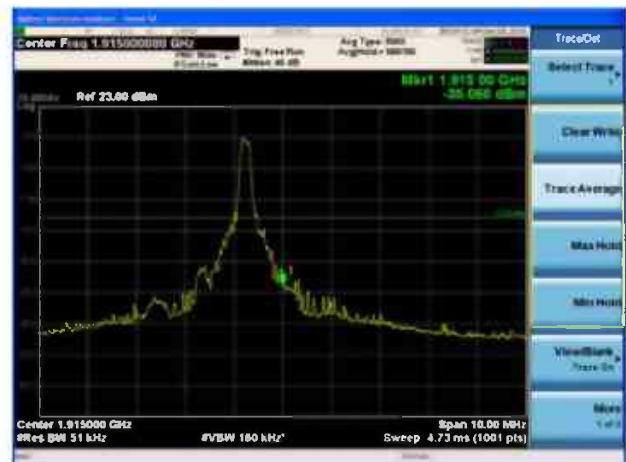
LTE Band 25 10MHz QPSK 100%RB CH-High
