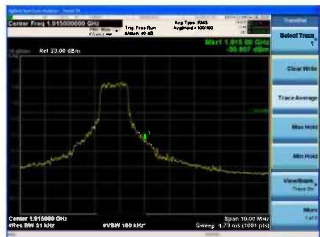
LTE Band 25 15MHz QPSK 1RB CH-High
