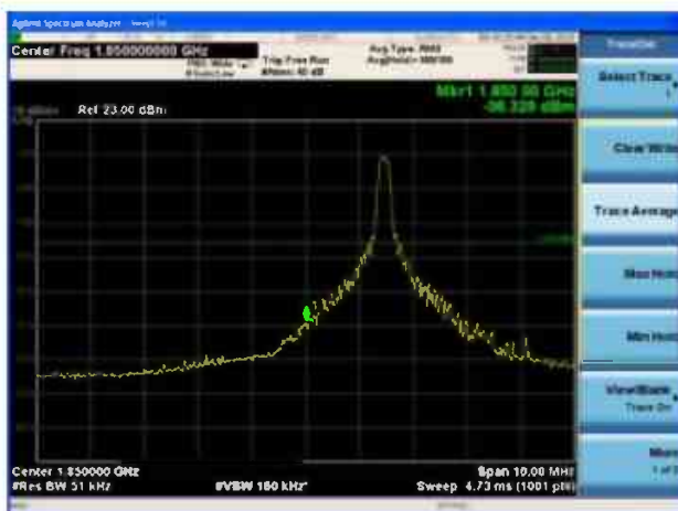
LTE Band 25 20MHz QPSK 100%RB CH-Low
