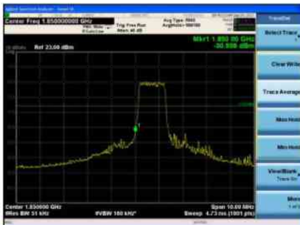
LTE Band 2 3MHz QPSK 1RB CH-Low
