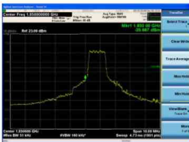
LTE Band 25 5MHz QPSK 100%RB CH-Low
