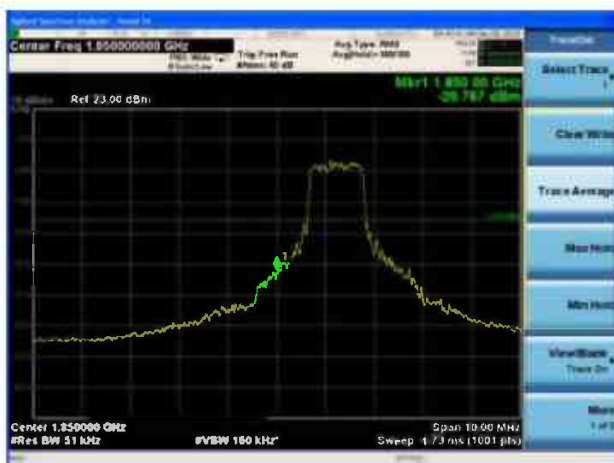
LTE Band 25 15MHz QPSK 1RB CH-Low
