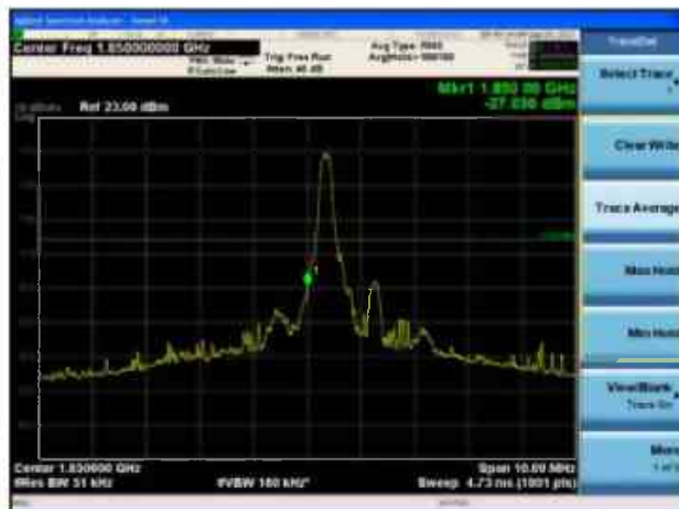
LTE Band 2 5MHz 16QAM 100%RB CH-Low
