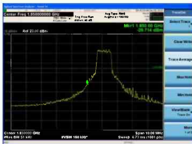
LTE Band 25 15MHz 16QAM 1RB CH-Low
