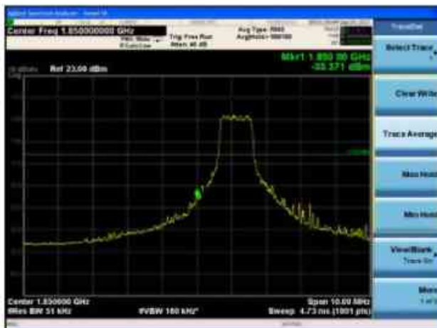
LTE Band 2 15MHz 16QAM 1RB CH-Low
