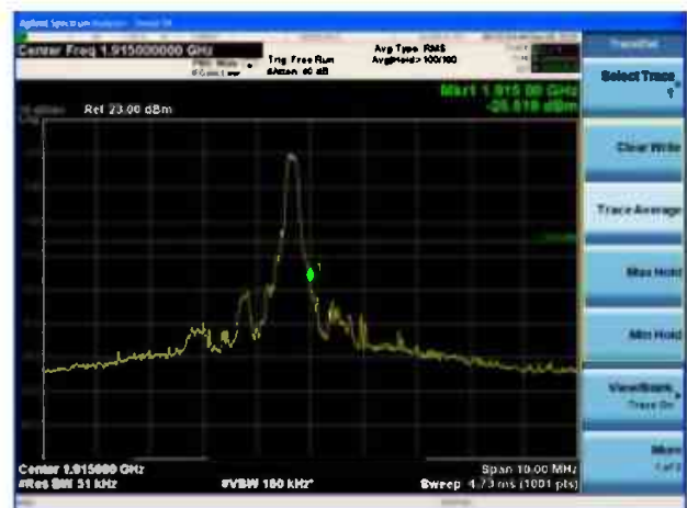
LTE Band 25 5MHz QPSK 100%RB CH-High
