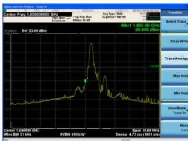
LTE Band 25 3MHz 16QAM 1RB CH-Low
