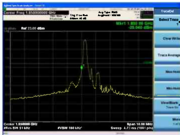
LTE Band 25 1.4MHz 16QAM 100%RB CH-Low
