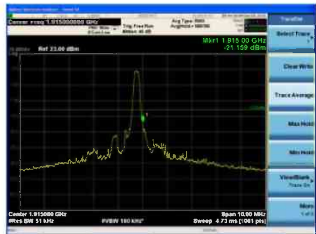
LTE Band 25 1.4MHz QPSK 100%RB CH-High
