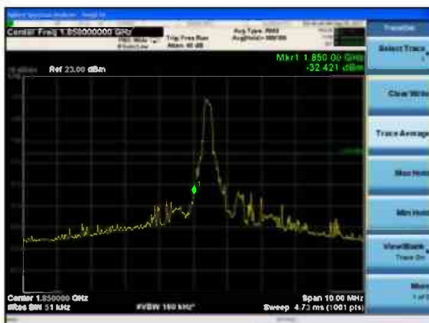
LTE Band 2 3MHz 16QAM 100%RB CH-Low
