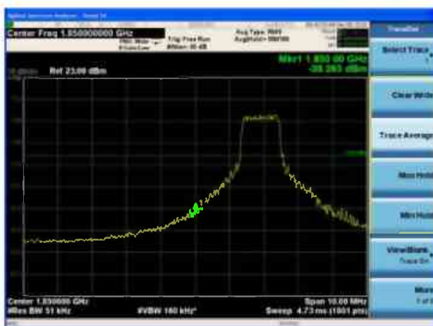
LTE Band 25 20MHz QPSK 100%RB CH-Low
