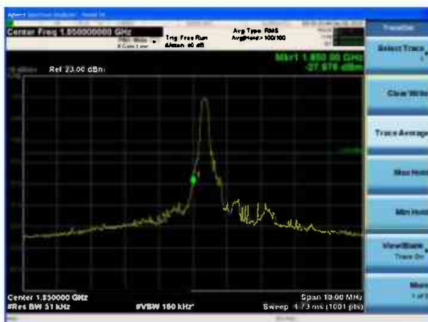
LTE Band 25 5MHz QPSK 100%RB CH-Low
