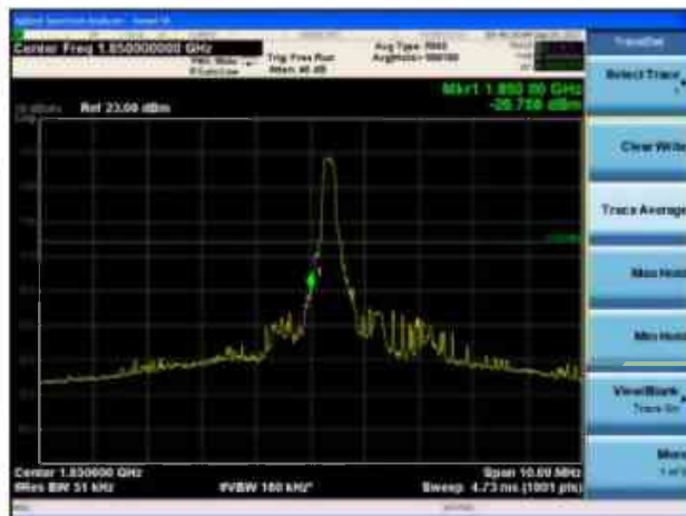
LTE Band 2 5MHz QPSK 100%RB CH-Low
