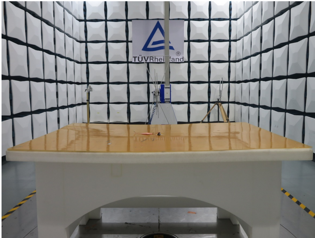
Photograph 1: Set-up for Radiated Spurious Emission, Below 1GHz
