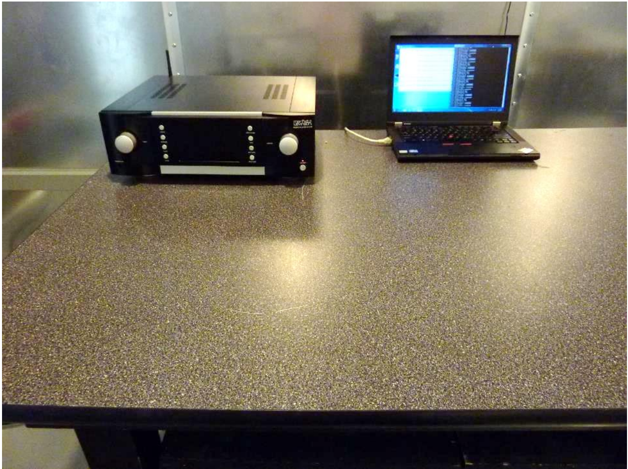
Figure 10: Conducted Emission Test Setup (Front)
