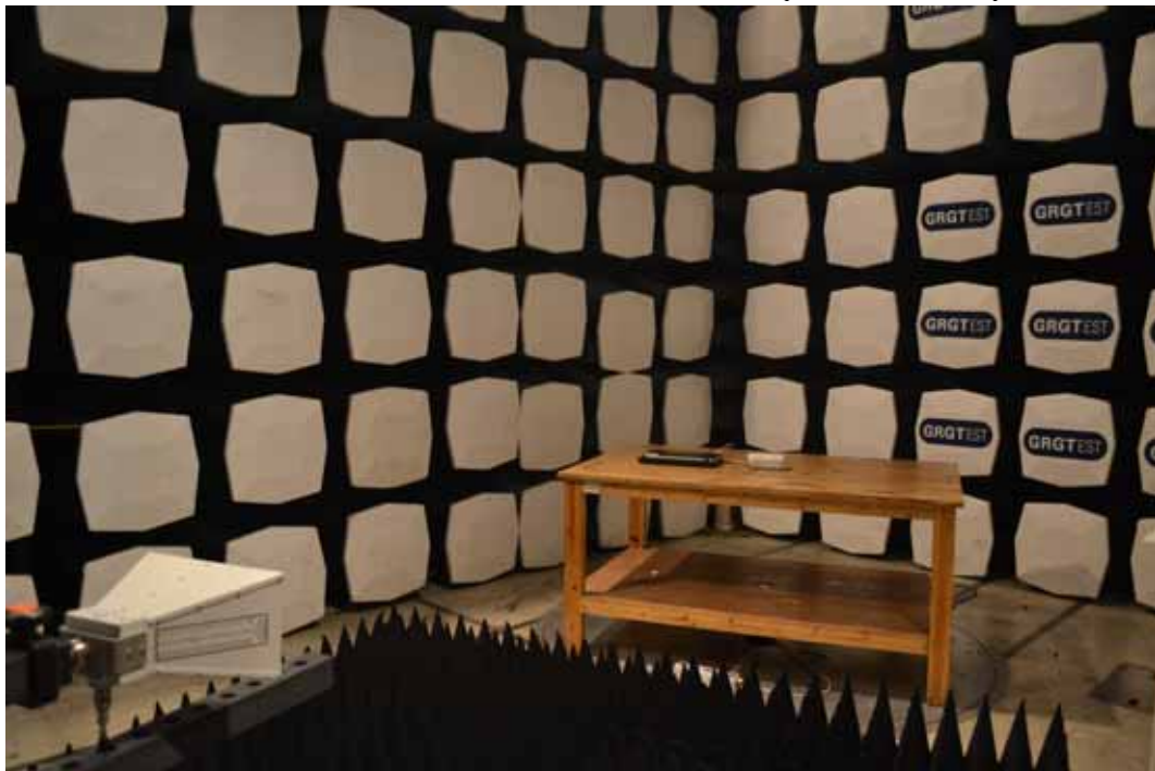
RADIATED SPURIOUS EMISSION TEST ( Above 1GHz )
