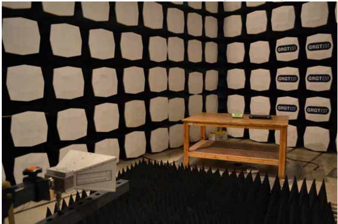
RADIATED SPURIOUS EMISSION TEST ( Above 1GHz )
