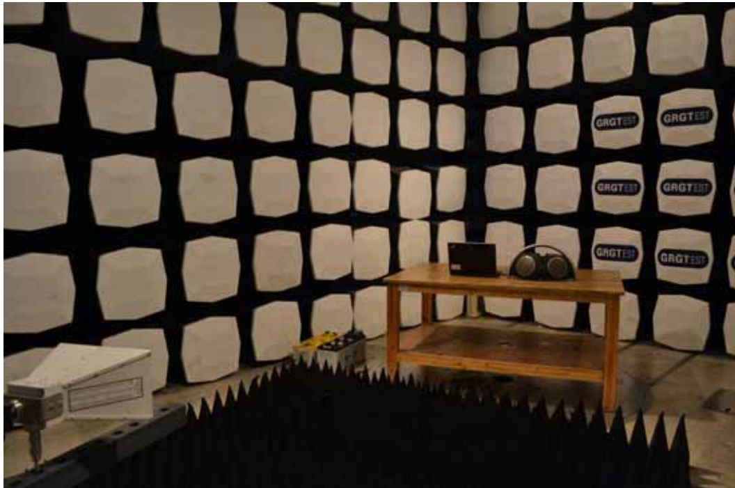
RADIATED SPURIOUS EMISSION TEST ( Above 1GHz )
