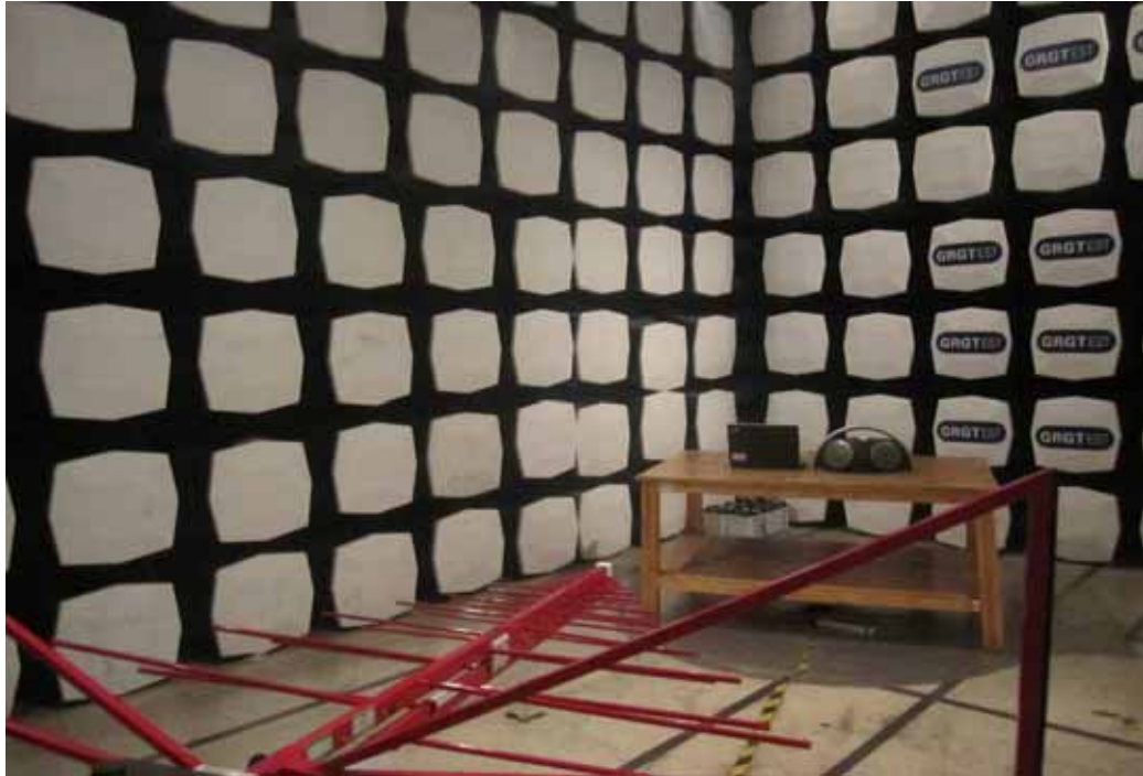
RADIATED SPURIOUS EMISSION TEST ( Below 1GHz )
