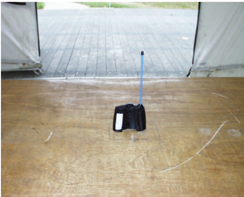
Radiated Open Site Test Set-up
