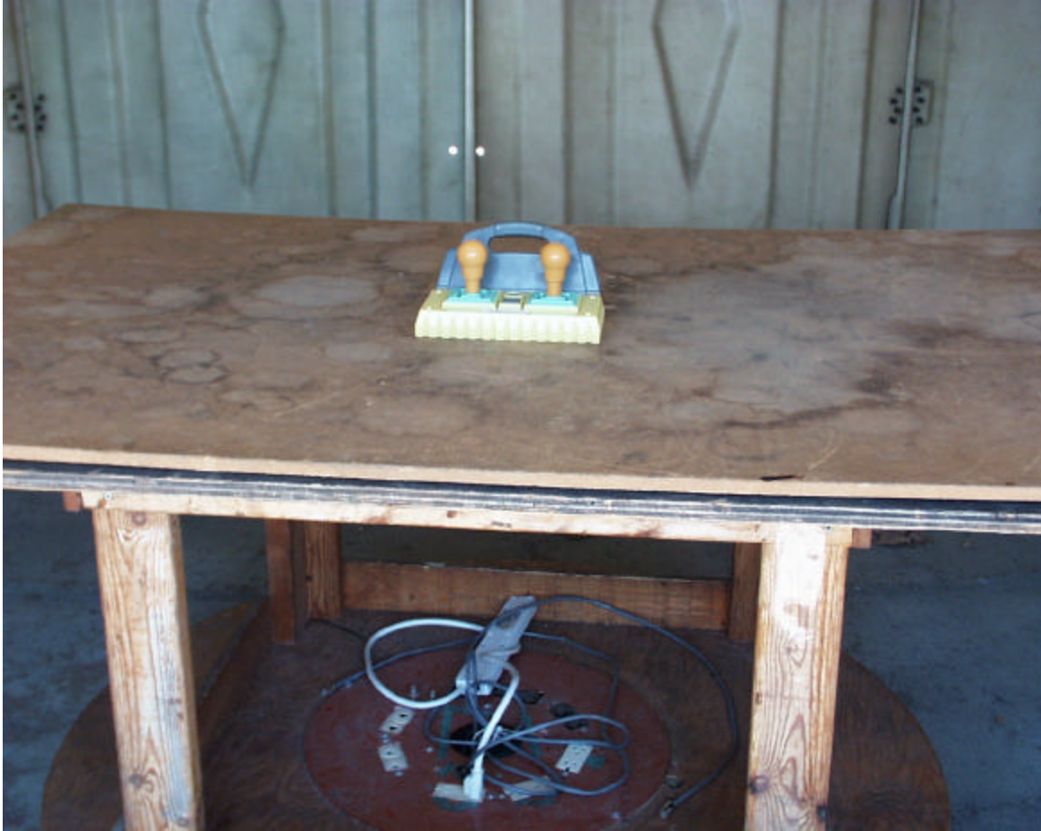
Radiated Open Site Test Set-up
