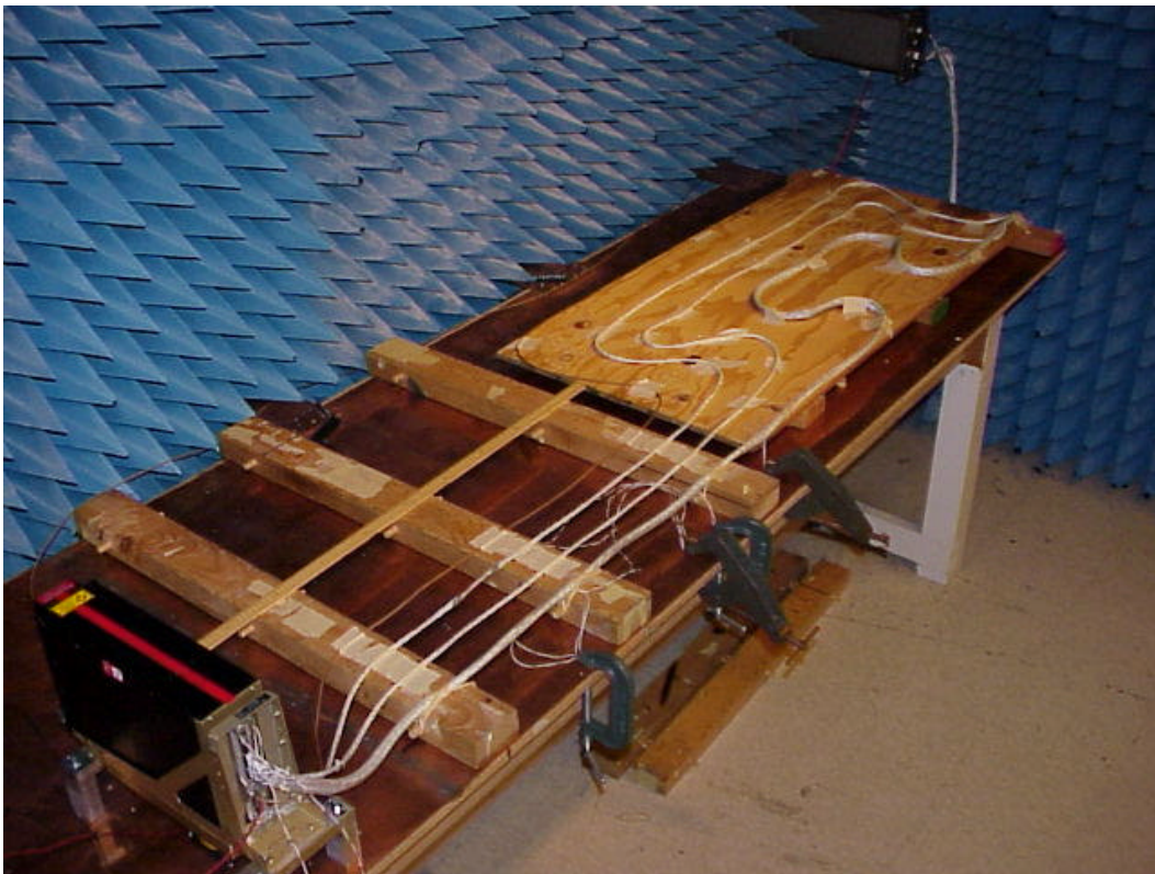
RTA-44D in EMI Test Chamber showing Interconnecting Cable Harness
