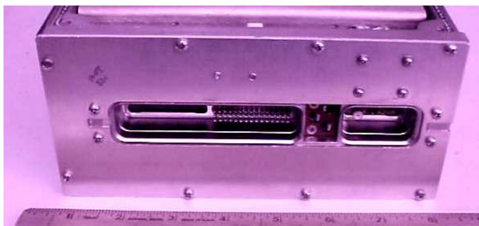
Rear Interconnect Module as part of LRU.
