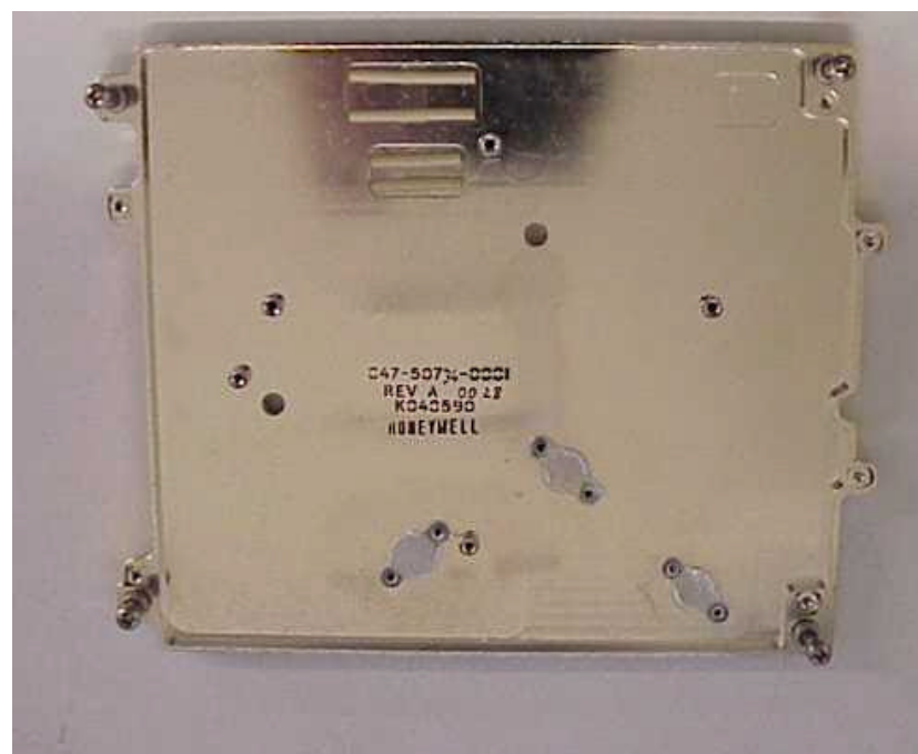
Bottom Side of Main RF Board with Heatsink (right) removed .
