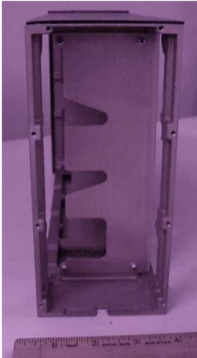
Rear Interconnect Module removed from LRU.
