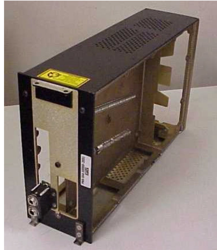
Remaining Chassis when all assemblies have been removed
