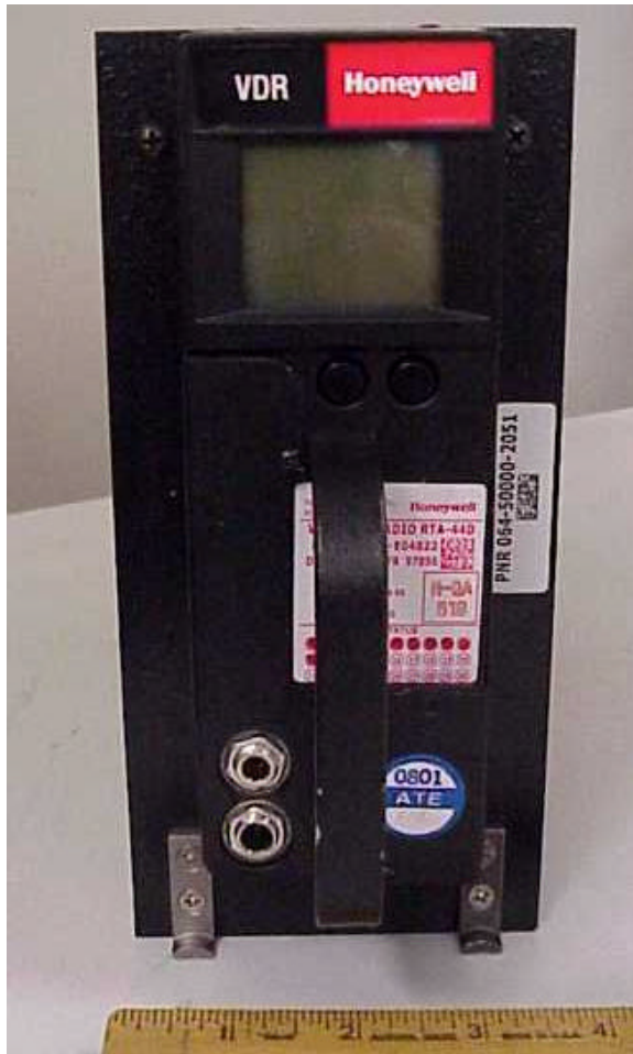
Front Panel Assembly as part of LRU (exterior front and interior views).
