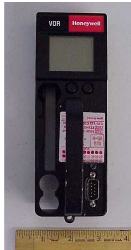
Front Panel Assembly with PCMCIA card slot and RS232 covers removed, and then the Front panel assembly removed from LRU chassis.
