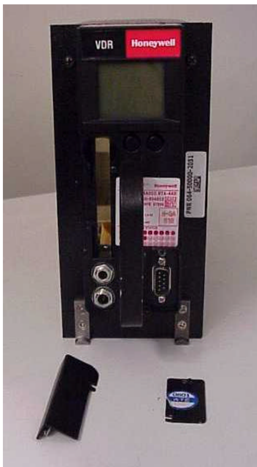
Front Panel Assembly with PCMCIA card slot and RS232 covers removed, and then the Front panel assembly removed from LRU chassis.
