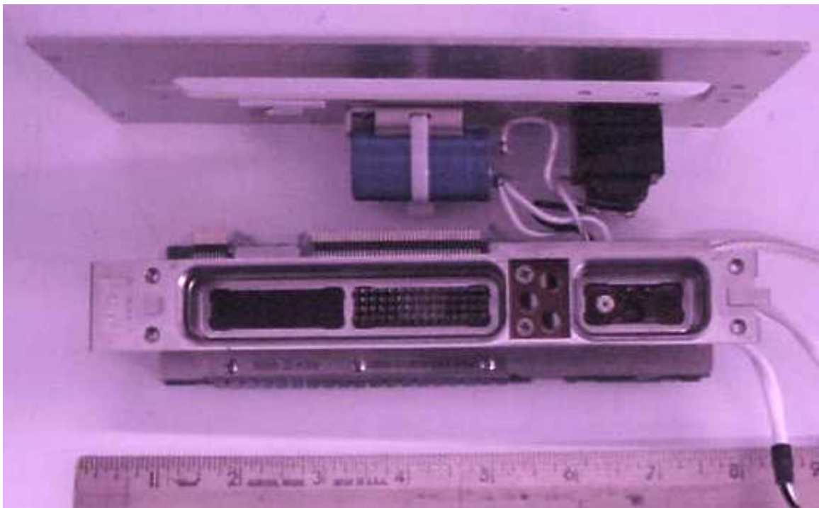
Cover and rear plate removed from Rear Interconnect Module.
