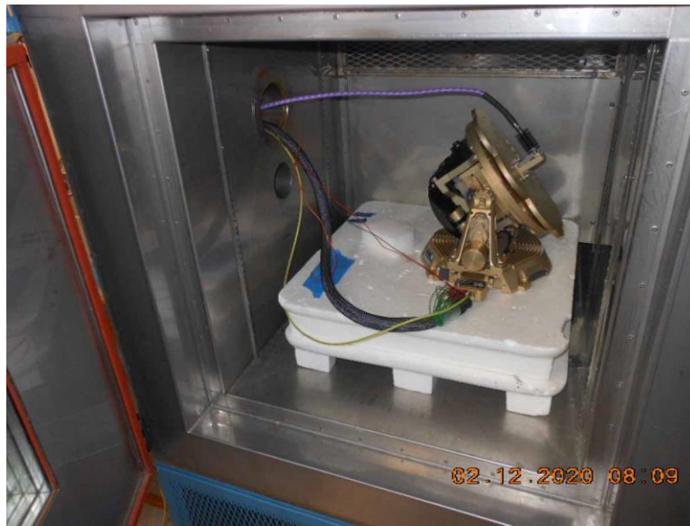
Temperature Chamber Setup, EUT
