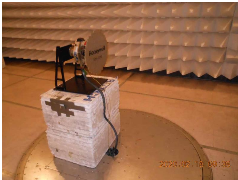
Radiated Test Setup 18inch
