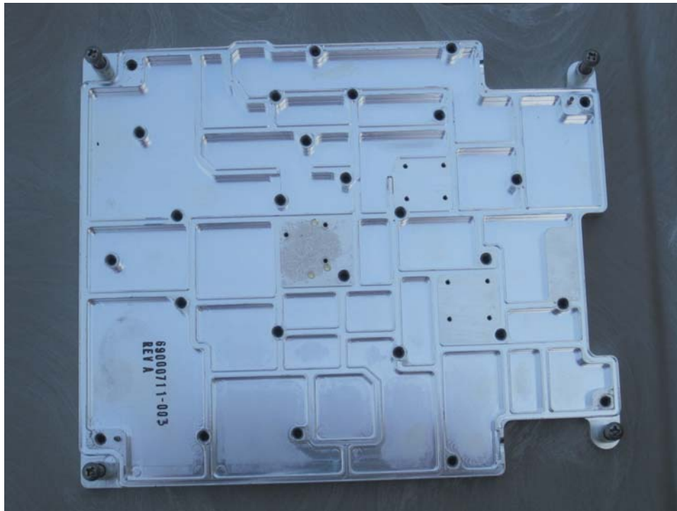
Shield Heatsink 1 with RF Board Removed
