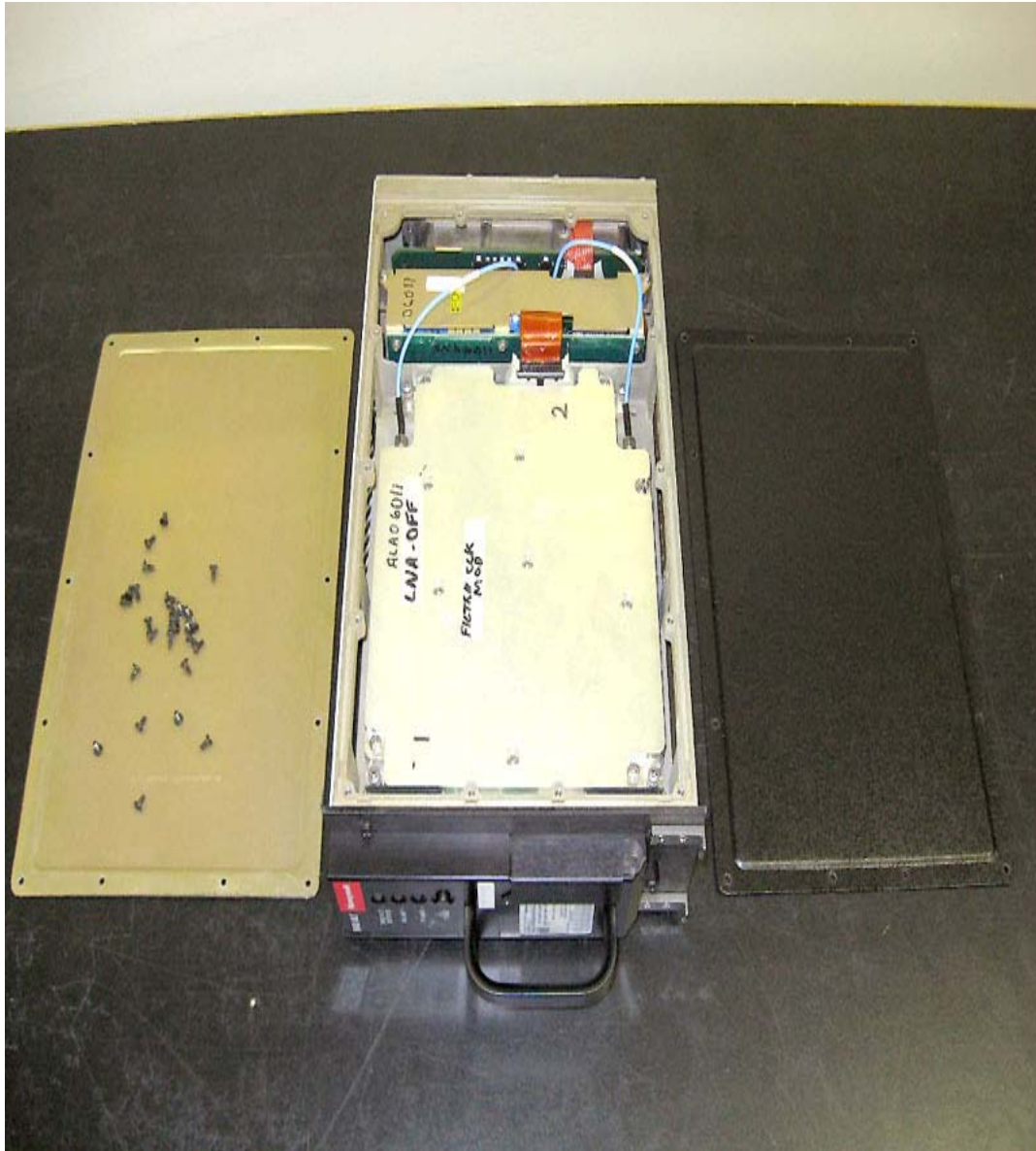
Submittal - Covers removed (RF board side)
