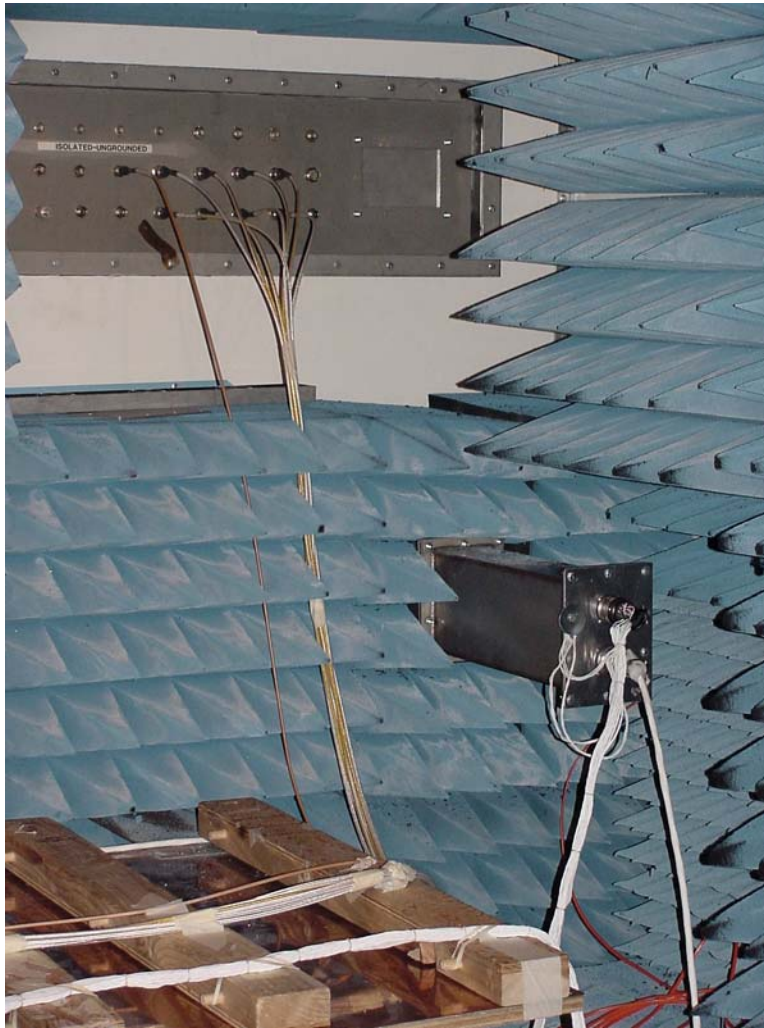
EMI Room test chamber showing TCAS harness breakout into control room.
