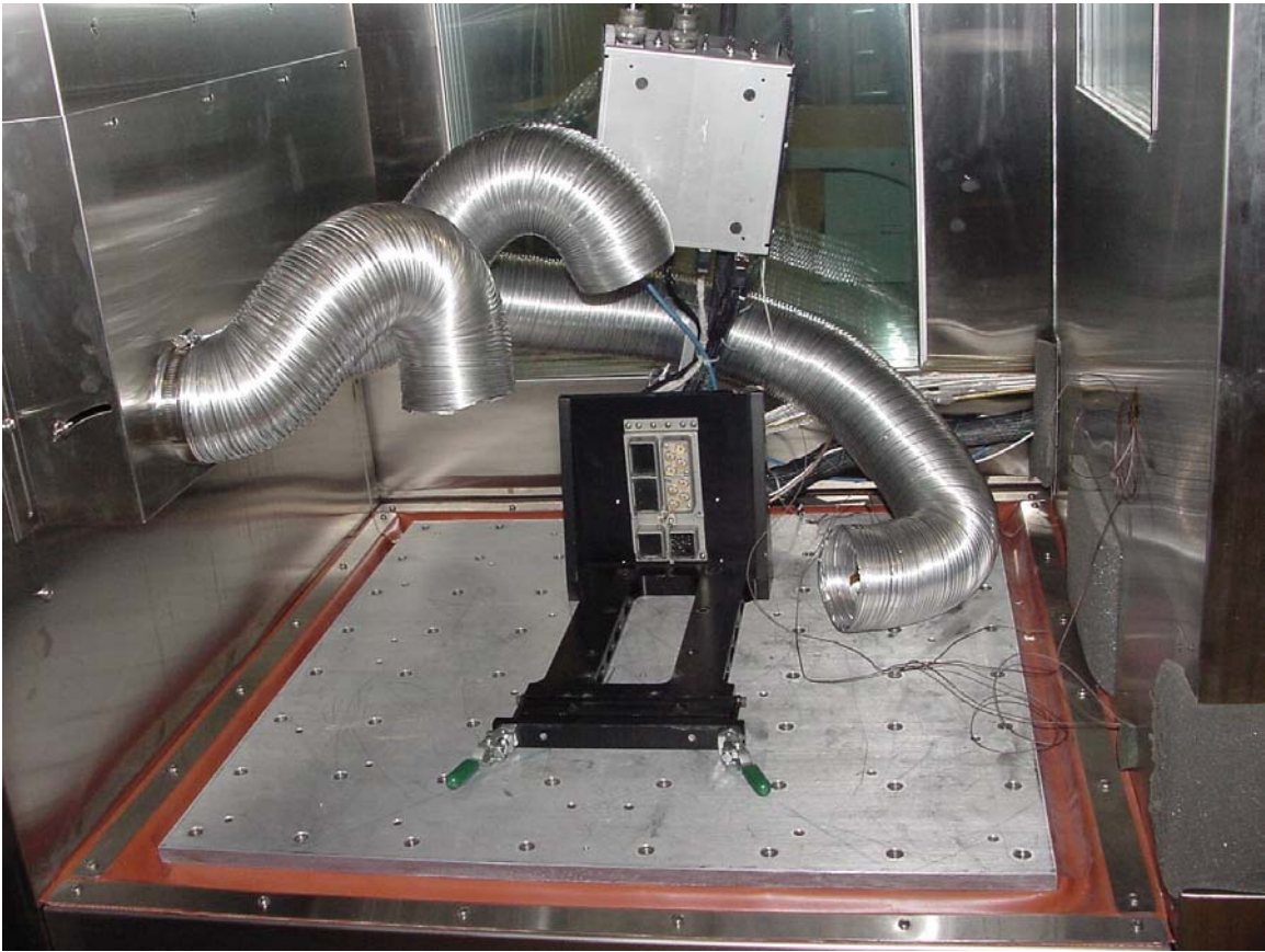
HALT Chamber (Highly Accelerated Life Test)
