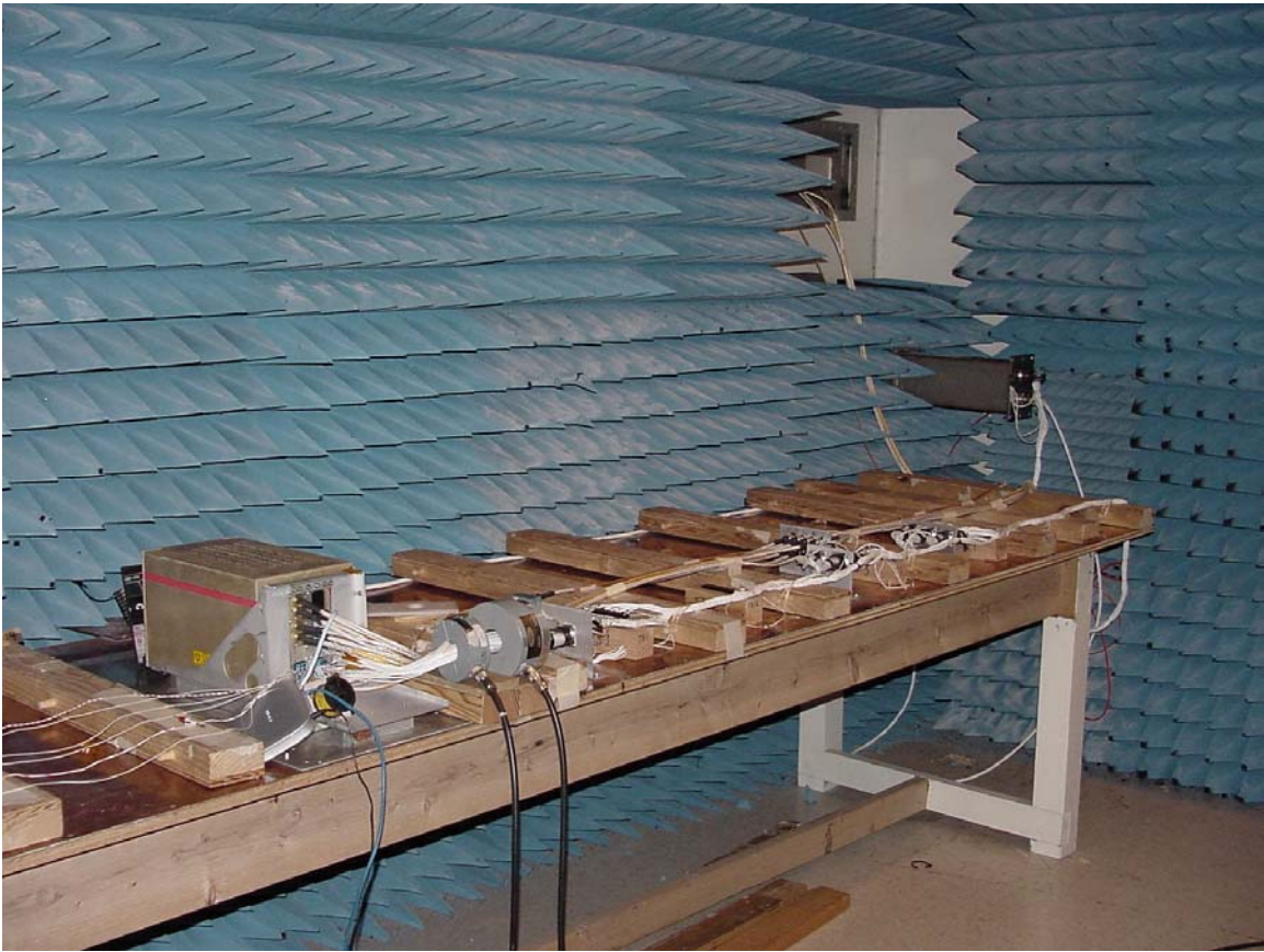
EMI Room test chamber showing TCAS harness.
