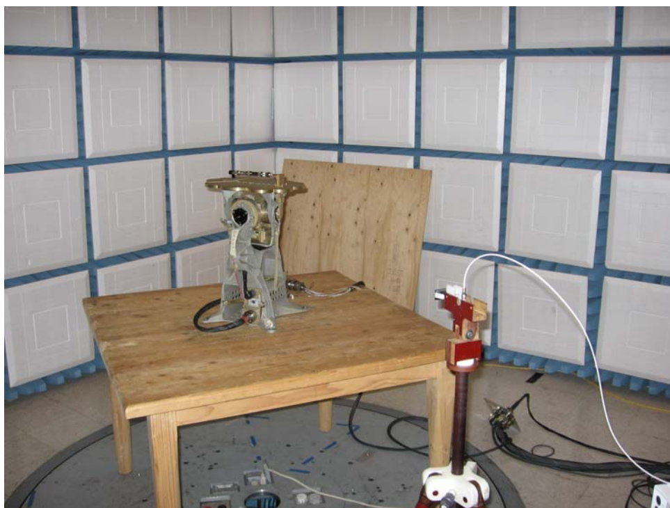
Figure 12-13 Field Strength Measurement 18 – 26 GHz
