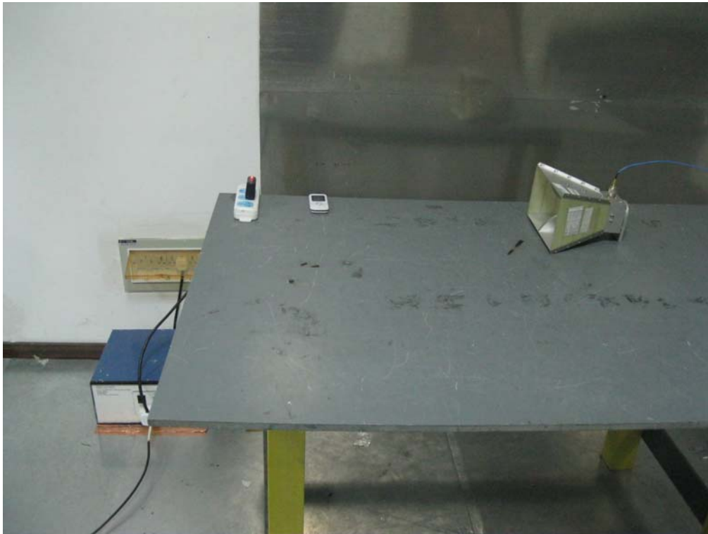
Conducted Emissions Test Setup - Front View
