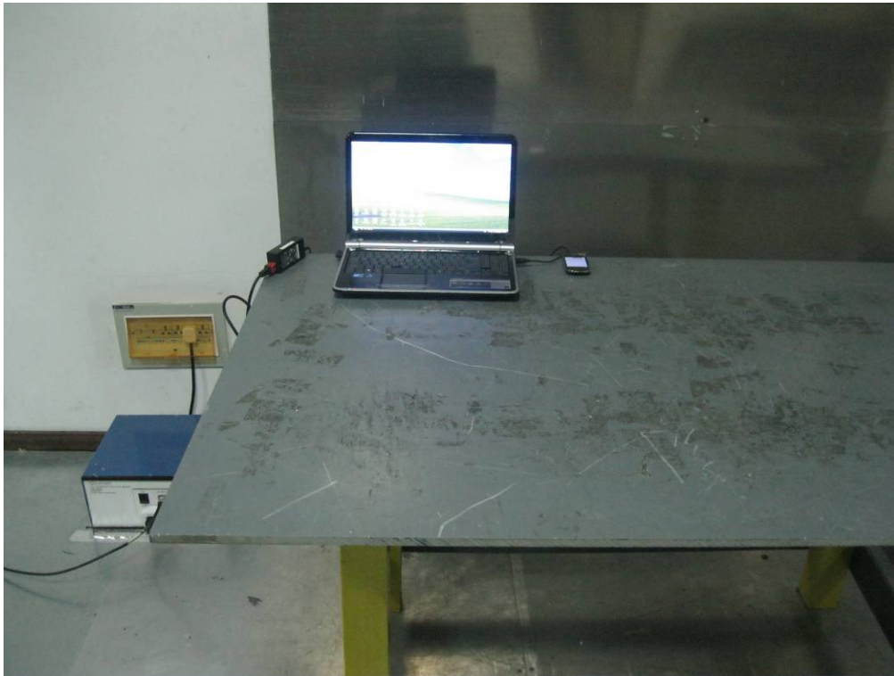
Conducted Emissions Test Setup - Front View
