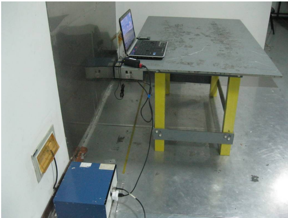
Conducted Emissions Test Setup - Side View
