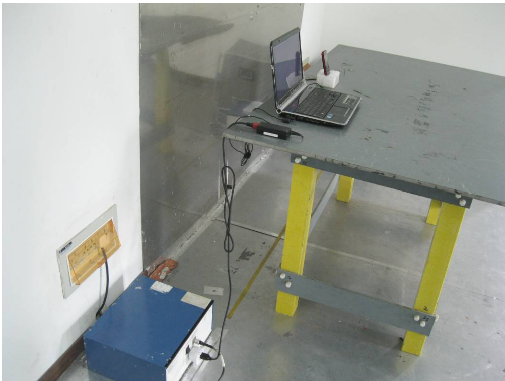
Conducted Emissions Test Setup - Side View
