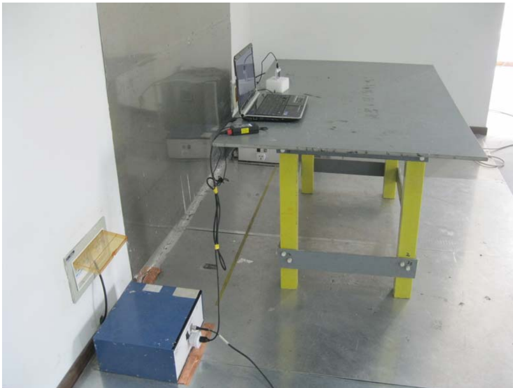
Conducted Emissions Test Setup - Side View
