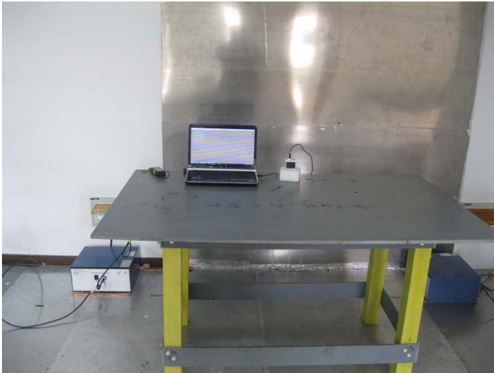
Conducted Emissions Test Setup - Front View
