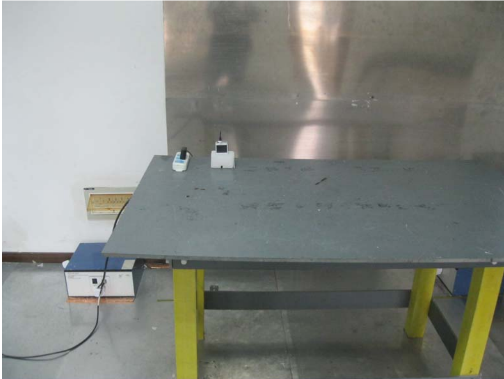
Conducted Emissions Test Setup - Front View
