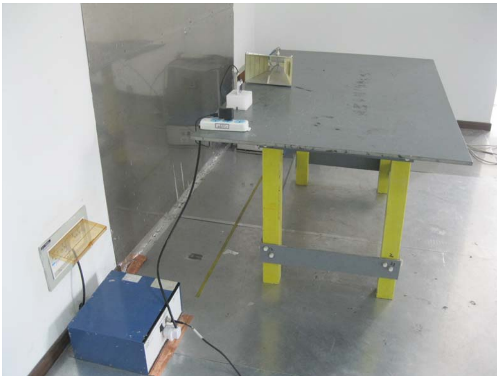
Conducted Emissions Test Setup - Side View
