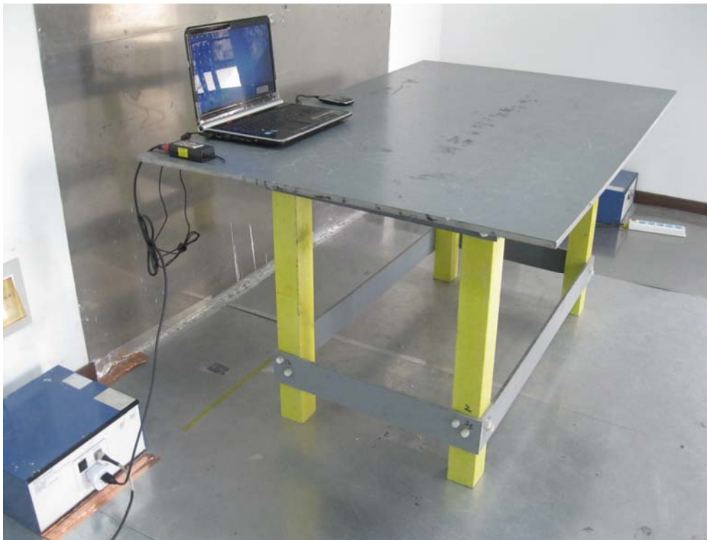
Conducted Emissions Test Setup - Side View
