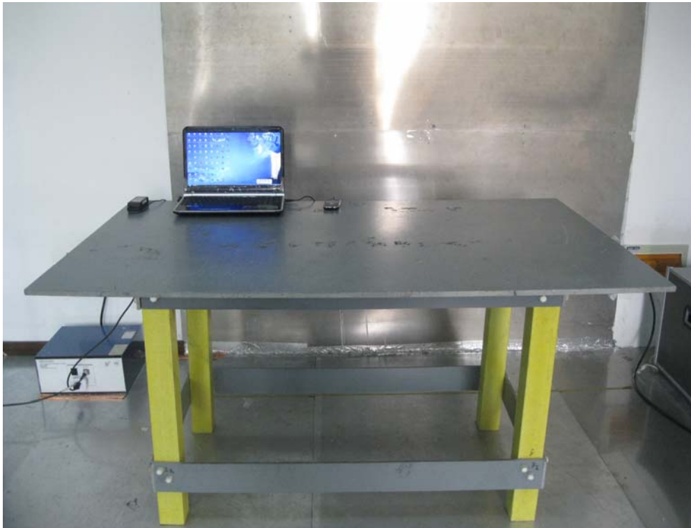
Conducted Emissions Test Setup - Front View
