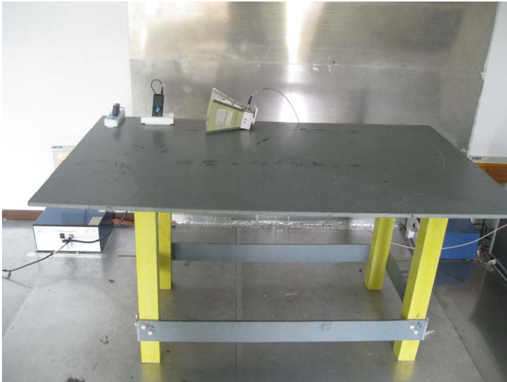
Conducted Emissions Test Setup - Front View
