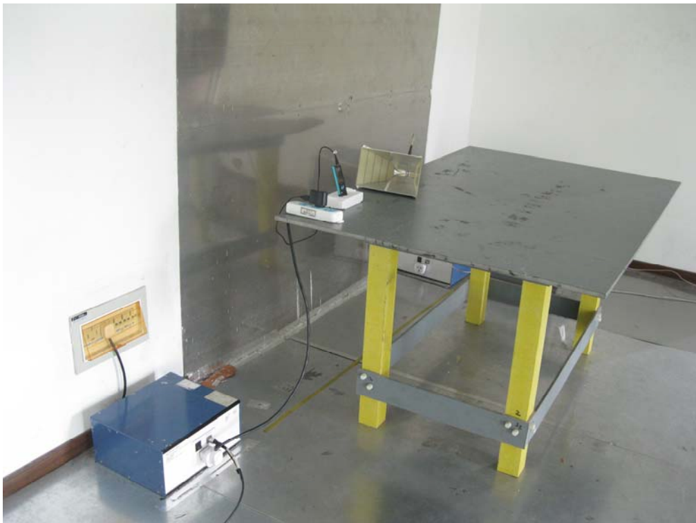
Conducted Emissions Test Setup - Side View
