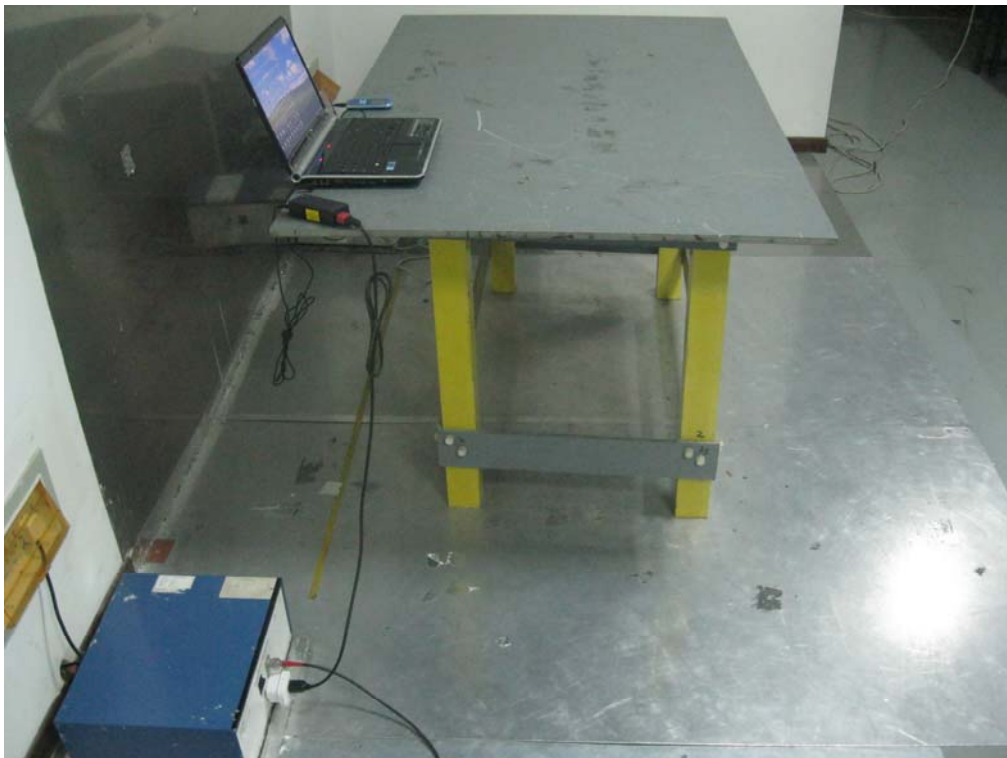
Conducted Emissions Test Setup - Side View
