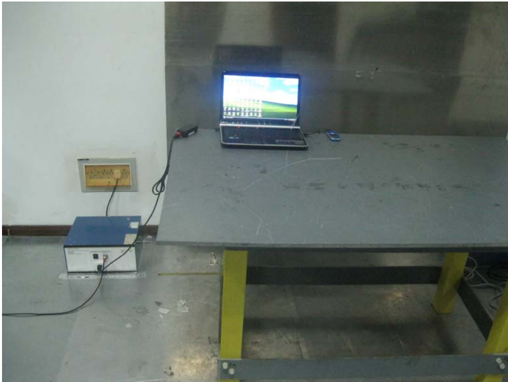
Conducted Emissions Test Setup - Front View
