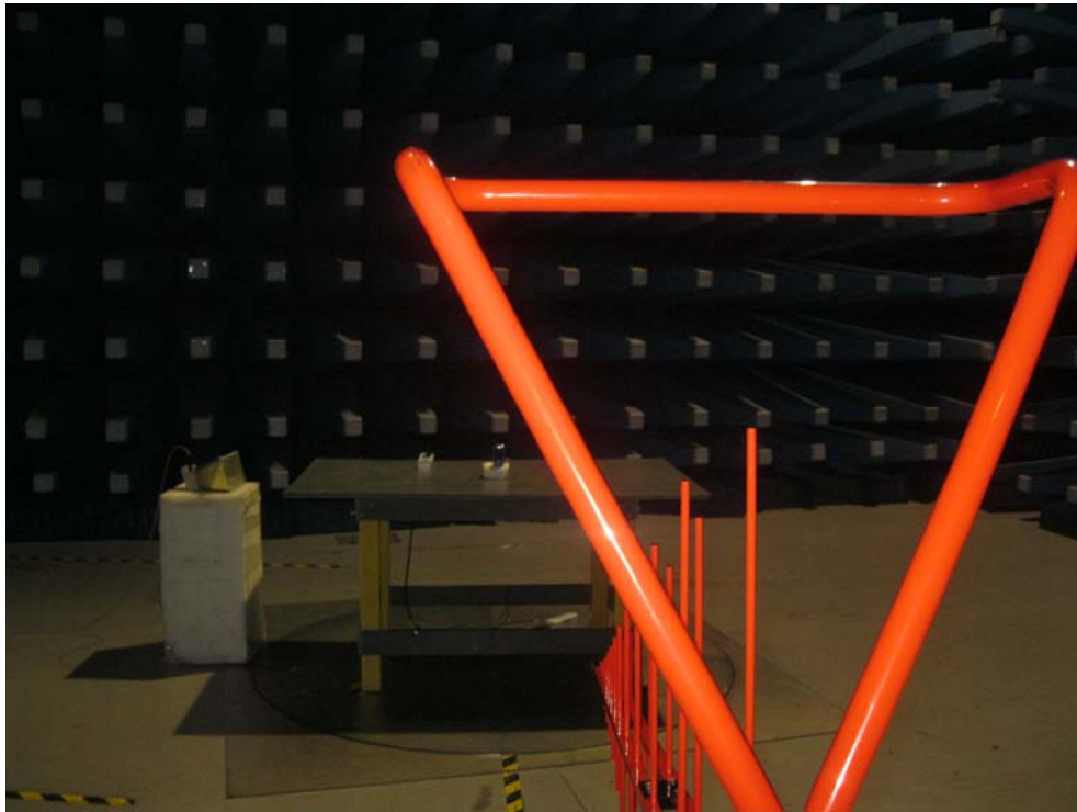
adiated Spurious Emissions Test Setup Below 1GHz - Front View
