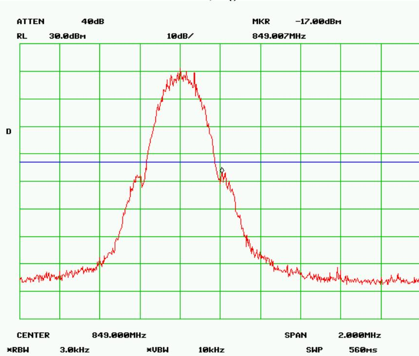
Note: offset= cable loss + 10log(1%\*26dB/3kHz)
