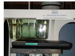
Figure 13.1 11 MBps BODY SAR Test Setup
