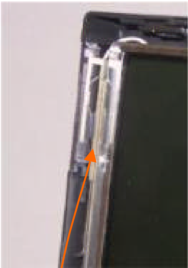
Left side antenna Inverted-F type Tx/Rx switching
