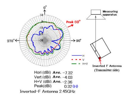
Therefore the peak radiated (EIRP) output power is calculated as follows.
