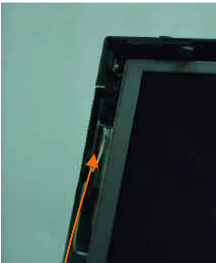
Left side antenna ( Inverted-F type ) WLAN only : Tx / Rx
