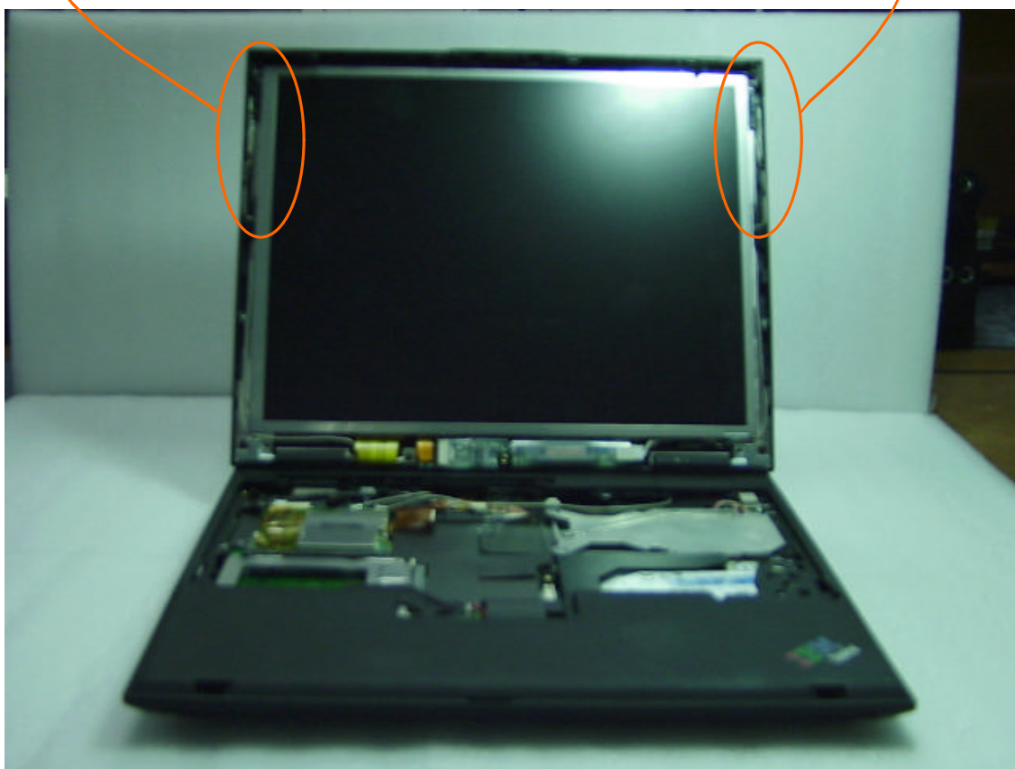
Left side antenna Inverted-F type Tx/Rx switching
