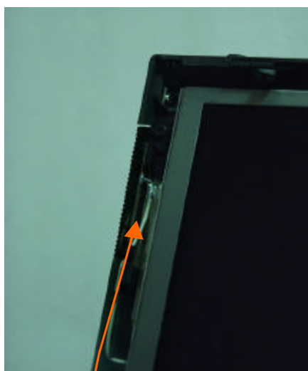
Left side antenna Inverted-F type Tx/Rx switching
