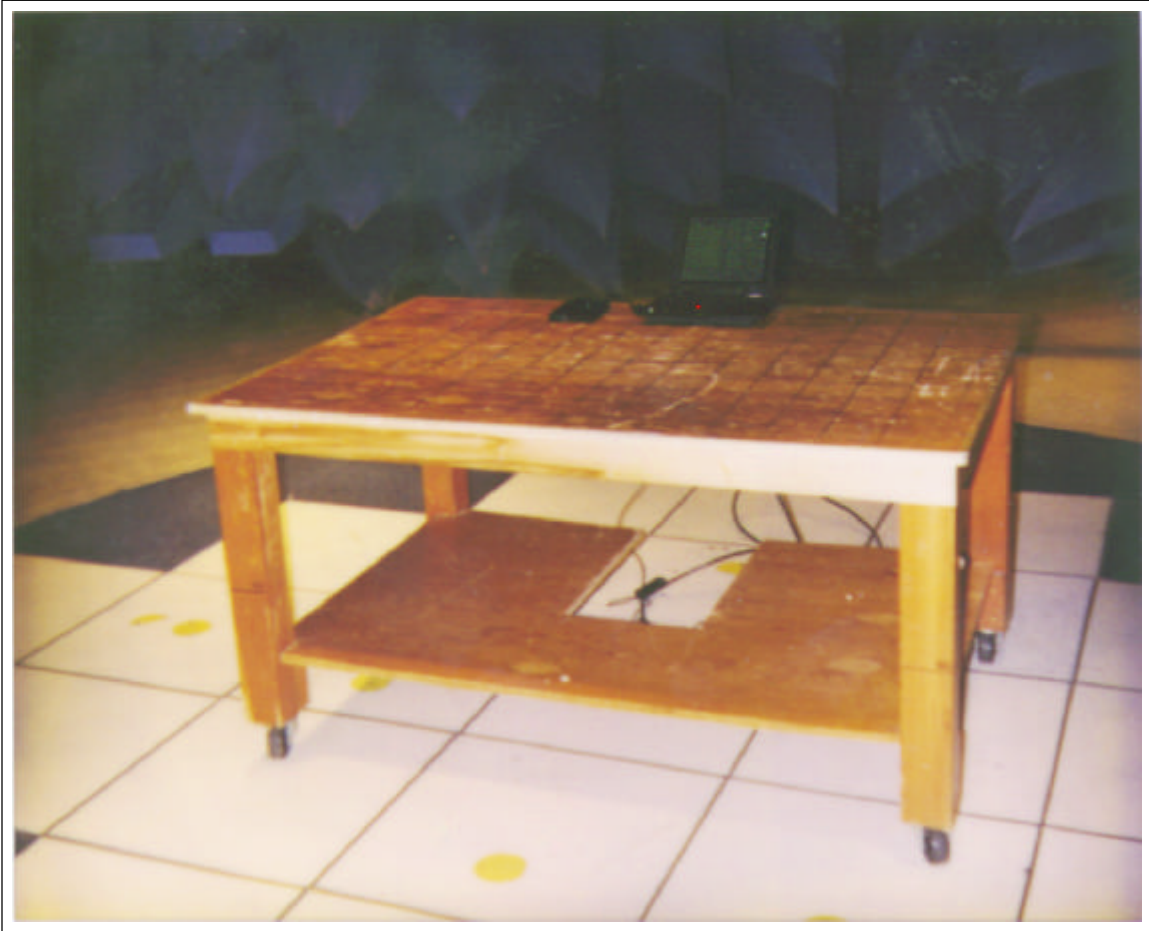
Front View Radiated Emissions Photograph Showing the EUT Configuration for Maximum Emissions
