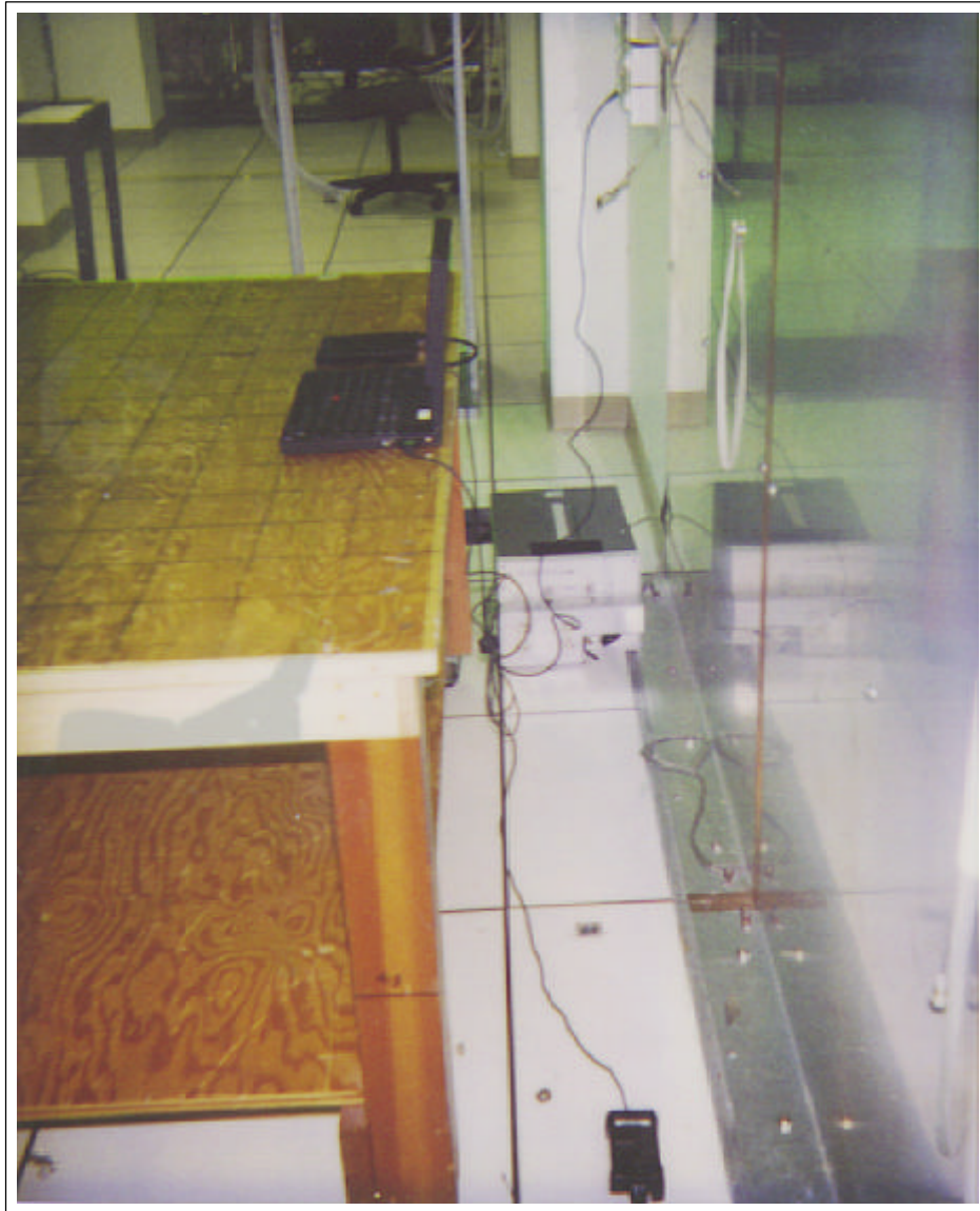
Rear View Conducted Emissions Photograph Showing the EUT Configuration for Maximum Emissions
