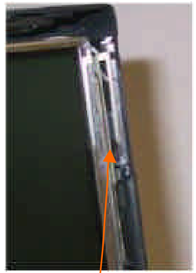
Right side antenna Inverted-F type
