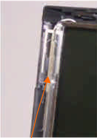
Left side antenna Inverted-F type
