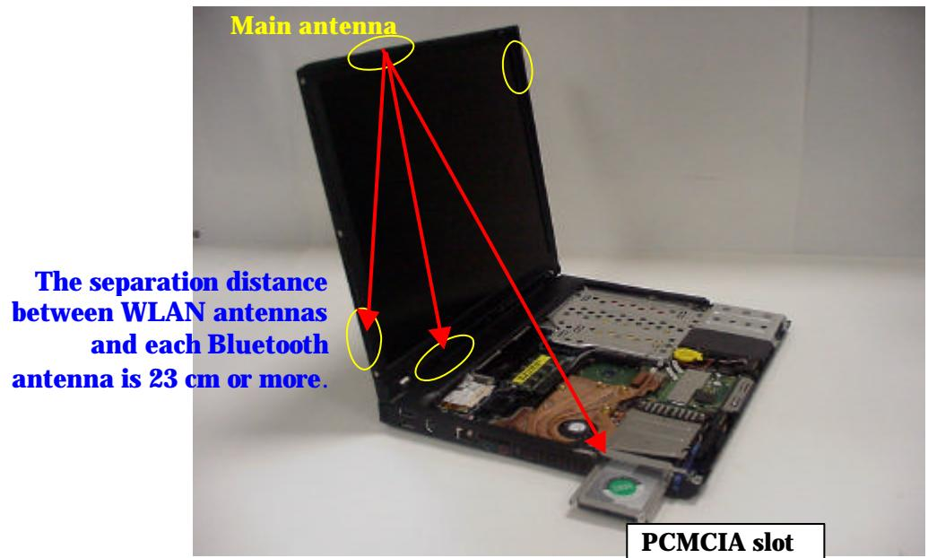
The main and auxiliary antennas located at LCD section of each host device (ThinkPad T40 Series, or R50 Series) are assembled apart from each Bluetooth antenna shown in the previous pages with 20 cm or more.
