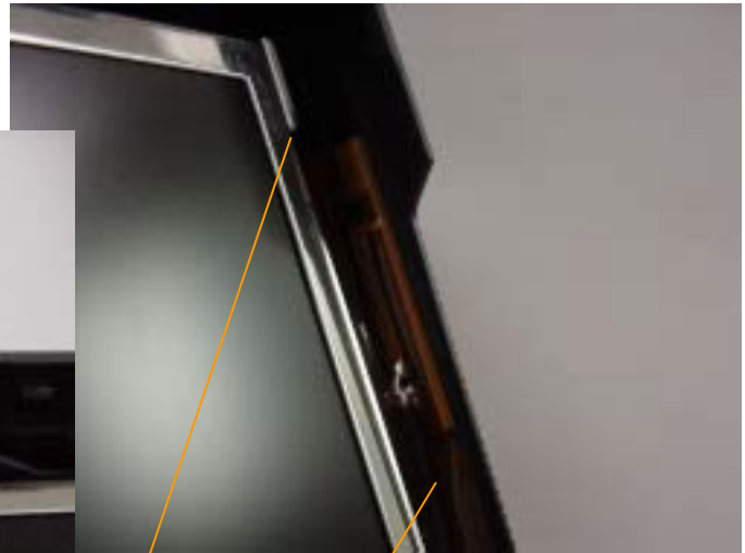
Auxiliary antenna Dual Band Inverted-F type
