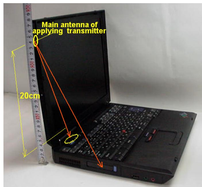
The main and auxiliary antennas placed at LCD section of the host device (ThinkPad R40 Series) are assembled apart from each Bluetooth antenna shown in the previous page with 20 cm or more.
