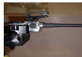
Figure 14.1 Body SAR Test Setup -- w/ Belt Clip --
