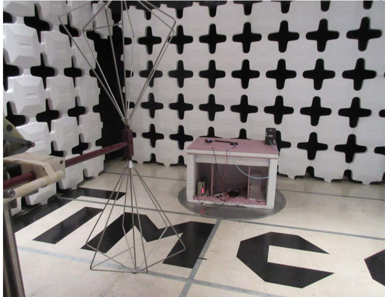
FIELD STRENGTH SPURIOUS EMISSIONS  $F < 1000\text{MHz}$
