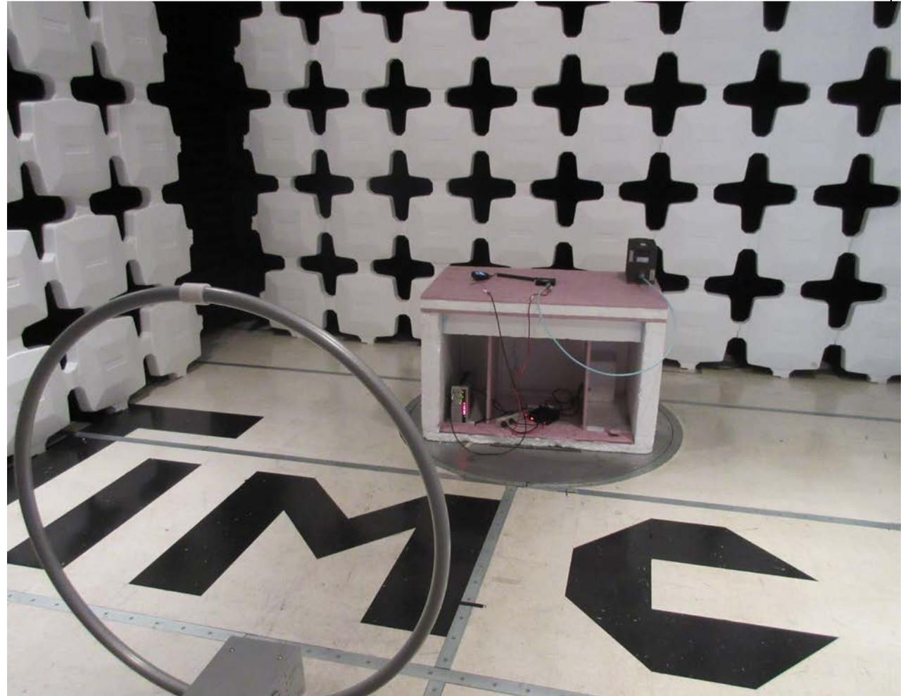
FIELD STRENGTH SPURIOUS EMISSIONS  $F < 200\text{MHz}$
